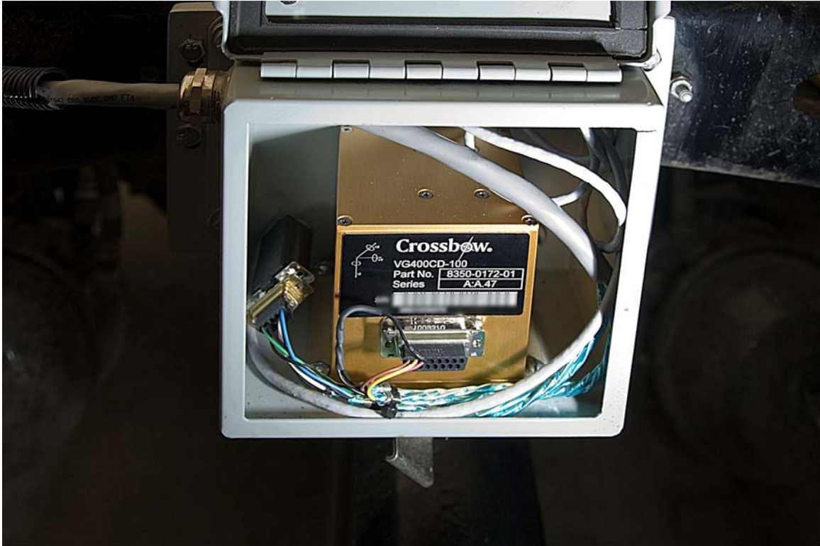
Figure 3-7. Rate Gyro and Accelerometer Enclosure (opened)
