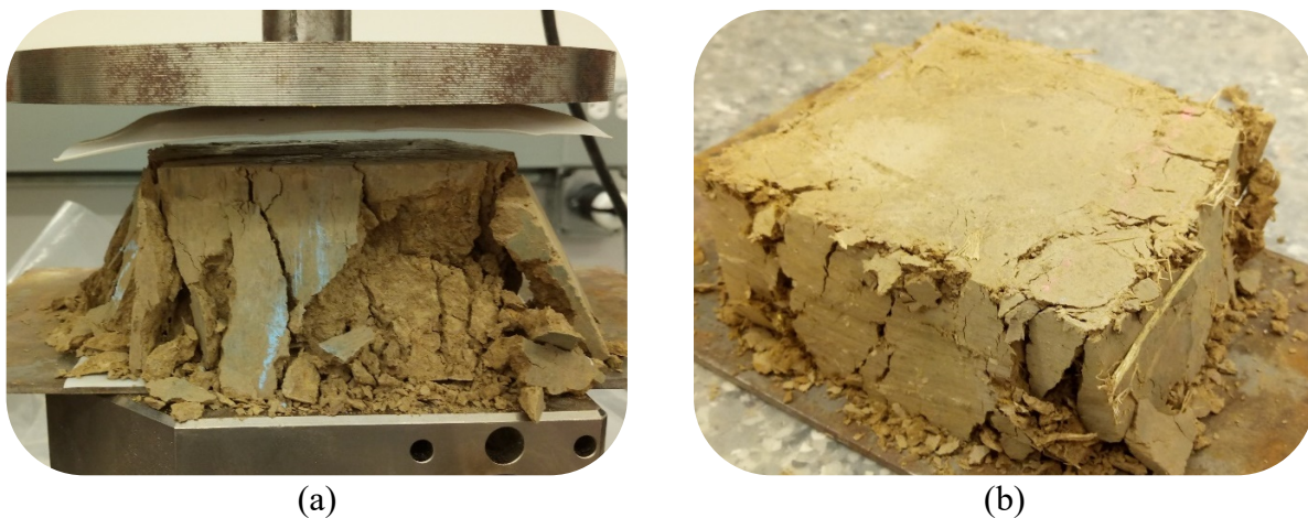
Figure 3.8. Failure under direct dry compression test: (a) EB-12-00 and (b) EB-12-05.
