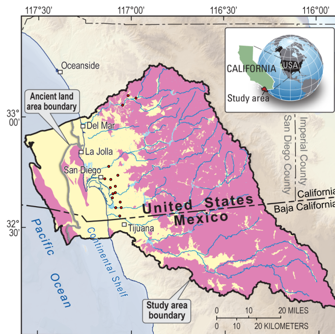
Fig. 3.1: Map illustrating the USGS San Diego Hydrogeology project study area, which extends offshore of San Diego. Sedimentary deposits are shown in yellow; hard rock is shown in pink; streams and water bodies are shown in blue; USGS monitoring-well sites are indicated by red dots (US Geological Survey 2021)
