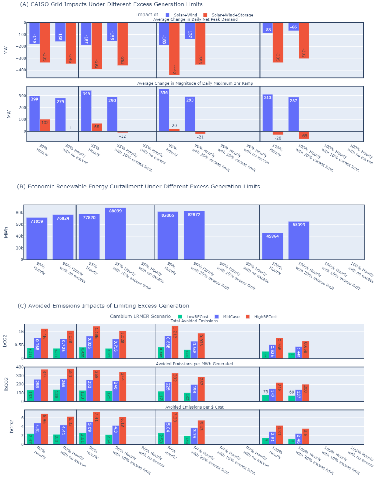
Figure 3.11 The impact of limiting excess generation on CAISO system peak and ramp needs (A), economic renewable energy curtailment (B), and avoided emissions (C).
