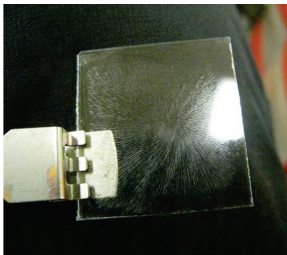
Figure 2.2 Spin-coated ZnO NP film on a glass substrate with the ZnO-methanol solution
