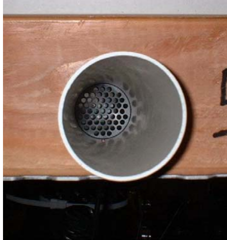
Figure 5. End view of calibrated boot leak showing the PVC plug with multiple small holes
