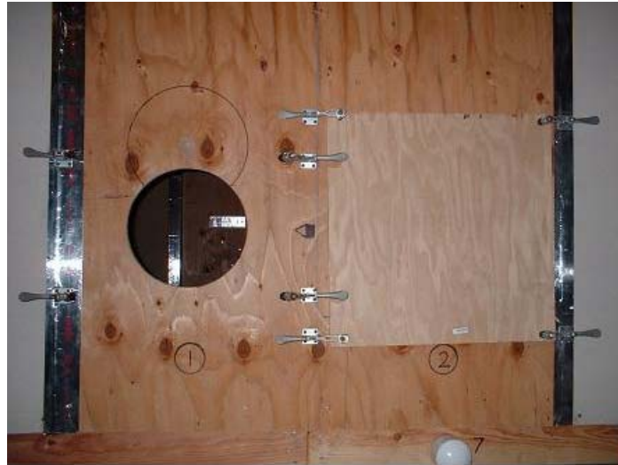
Figure 2. Test chamber hole number 1 open and hole number 2 with cover in place
