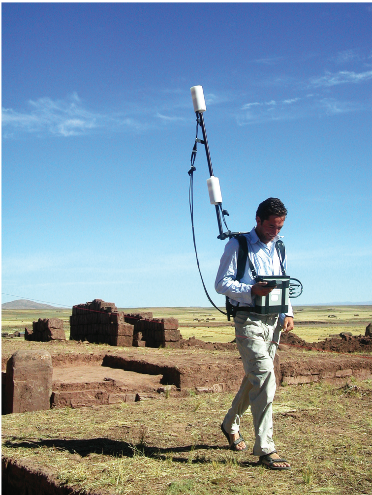
Figure 4.3 Magnetometry survey at Khonkho Wankane (photo by John W. Janusek).
