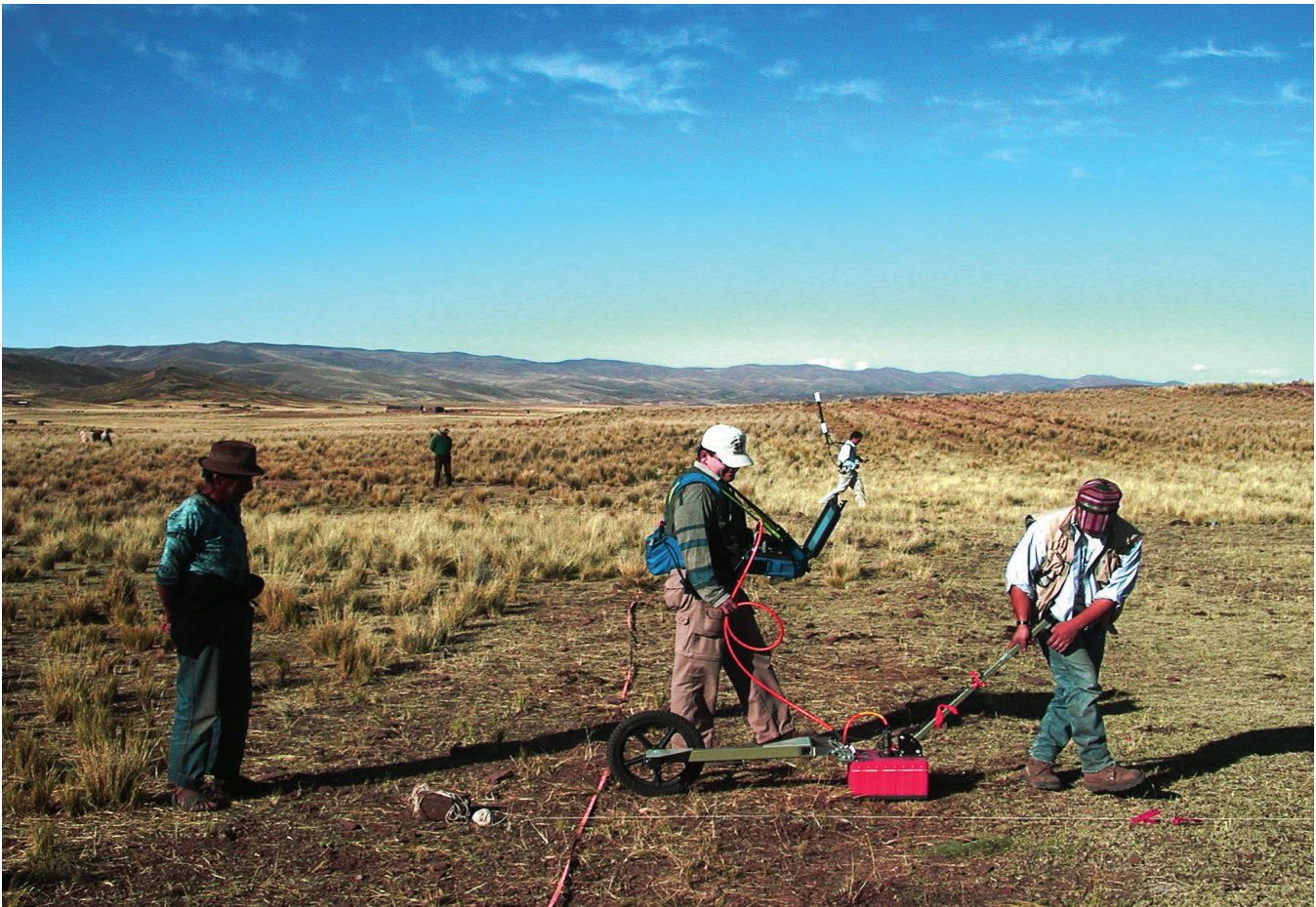
Figure 4.1 Ground Penetrating Radar survey at Khonkho Wankane (photo by John W. Janusek).
