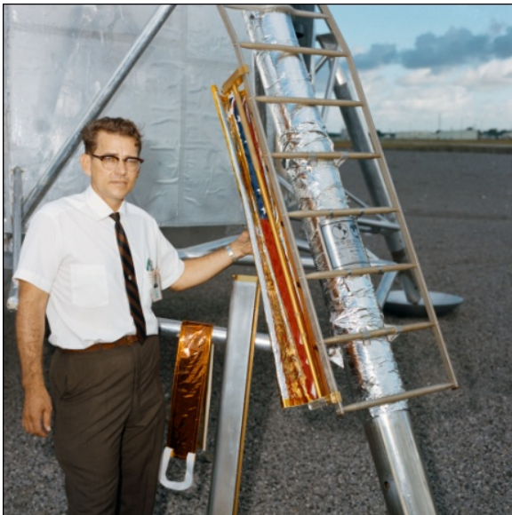
Figures 26–27: In the next steps of the deployment he removes the insulation from around the flag assembly (left) and then takes the flag from the mounting brackets (right). (NASA JSC Photos S69-38757, S69-38758).
