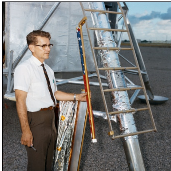
Figures 26–27: In the next steps of the deployment he removes the insulation from around the flag assembly (left) and then takes the flag from the mounting brackets (right). (NASA JSC Photos S69-38757, S69-38758).
