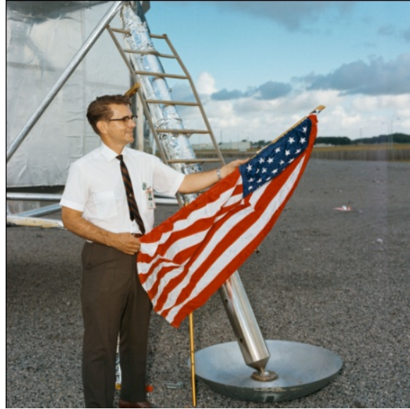
Figures 28–29: Next, the engineer shows the two parts of the lunar flag assembly—the lower pole, and the upper pole with the flag folded around it (left). He then extends the telescoping crossbar (right). (NASA JSC Photos S69-38759, S69-38760).
