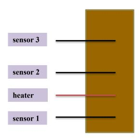
**Figure 1.** A diagram to illustrate probe placement. Sensor 1  $(x_1)$  is -0.75 cm upstream, and sensors 2  $(x_2)$  and 3  $(x_3)$  are 0.75 and 2.25 cm downstream from the heater, respectively.
