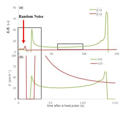
**Figure 3.** The ratio of temperature rises,  $\delta_2/\delta_1$  and  $\delta_3/\delta_2$ , between sensors,  $x_2/x_1$  and  $x_2/x_3$ , (a) are used to calculate velocities  $V_{12}$  and  $V_{23}$  (b). The time window in which the ratios are calculated (small box) and traces of the random noise errors that can occur following a heat pulse (large box).
