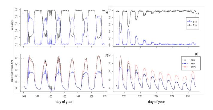
**Figure 5.** Diurnal patterns of the measurement uncertainties ( $\sigma_{12}$  and  $\sigma_{23}$ ) for sensor pairs  $x_1$  and  $x_2$ , and sensors  $x_2$  and  $x_3$  (a,c), and sap velocities (b,d) calculated with the double-ratio (DRM), heat-ratio (HRM), and compensation heat-pulse methods (CHPM) during a week of high transpiration when water was not limiting (a,b) and low transpiration during water limited conditions (c,d) in 2016 for an illustrative tree.
