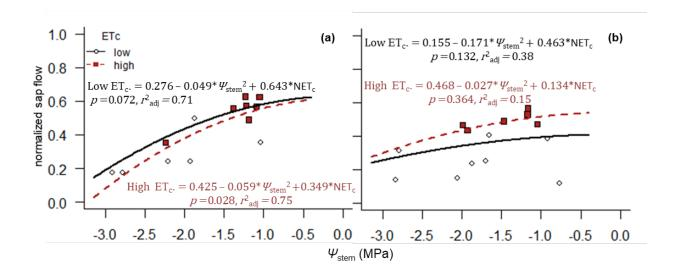
**Figure 8.** Relationship between midday stem water potential ( $\Psi_{\text{stem}}$ ) and normalized daily sap velocities, under high and low (above or below 6.8 mm d<sup>-1</sup>, respectively) ranges of crop evapotranspiration (ET<sub>c</sub>) for all trees during (a) 2016 and (b) 2017, with corresponding regression model lines. Data are expressed as the mean of all trees per day.
