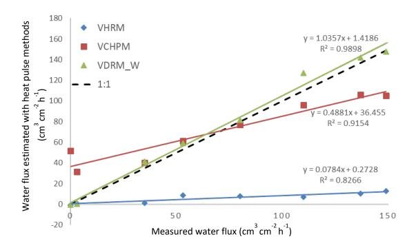
**Figure 4.** Results of the heat-ratio method (HRM), compensation heat-pulse method (CHPM), and double-ratio method (DRM) performance for calculating true gravimetric water flux in a sand-filled PVC pipe.
