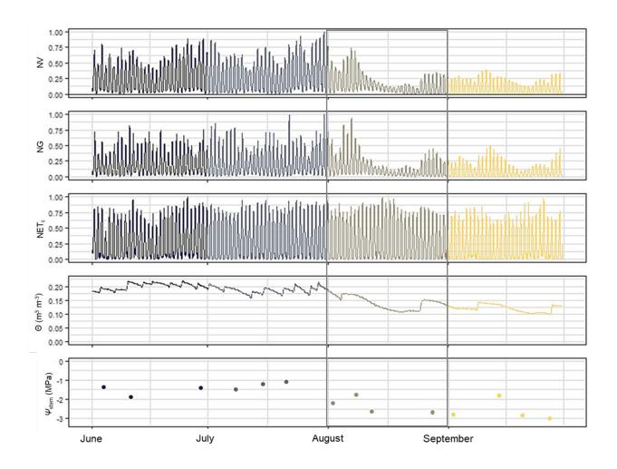
Figure 6. From the top to bottom panels: 2016 seasonal normalized sap velocity (NV) calculated using the double-ratio method, normalized isothermal canopy conductance (NG), normalized crop evapotranspiration (NET<sub>c</sub>), soil water content ( $\theta$ ), and midday stem water potentials ( $\Psi_{\text{stem}}$ ) in an illustrative tree at Nickels Soil Laboratory.
