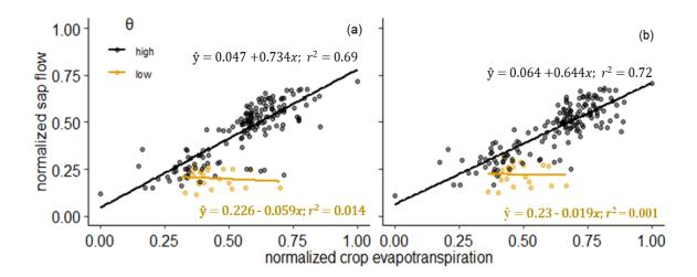
**Figure 7.** Averaged daily normalized sap velocity, calculated including (a) and excluding (b) nighttime data, as predicted by crop evapotranspiration at high (> 0.14 m<sup>3</sup> m<sup>-3</sup>, black lines and symbols) and low (< 0.14 m<sup>3</sup> m<sup>-3</sup>, tan lines and symbols) soil water content ( $\theta$ ) values. Data shown here exclude harvest periods in August.
