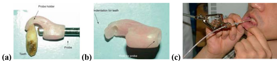
Fig. 1 Prototype intra-oral imaging probe holder. a The probe location is accurately controlled by its placement through a slot within the probe body. b The custom fabricated probe body is reproducibly fixated through a custom groove fitting onto an adjacent tooth. c Prototype extra-oral imaging probe holder. To ensure reproducible re-imaging at exactly the same location during multiple imaging events and to minimize movement artifacts, a multi-joint imaging probe holder for OCT imaging was fabricated. (Figure: courtesy of J.H.B.)
