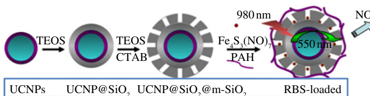
Scheme 4. Preparation of UCNP with a mesoporous silica shell impregnated with Roussin's black salt (red dots), a photoactive NO generator, and coated with poly(allylamine hydrochloride). NIR irradiation leads to upconversion to wavelengths overlapping the RBS absorbance and NO uncaging. (Online version in colour.)
