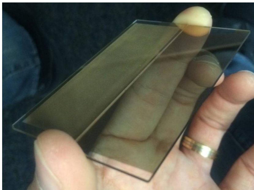
Figure 2.3.1: Glass slides plated with translucent gold
