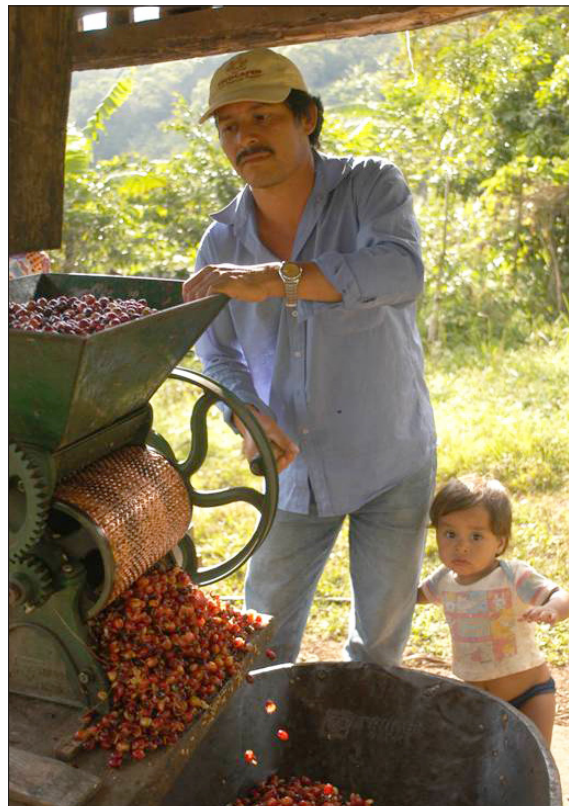
Segundo and his son depulp coffee at their small-scale family farm in San Ramon, Nicaragua. These small coffee mills offer an effective way to conserve water and keep the coffee pulp on the farm for making compost. (Photo by Bridget O'Brian)
