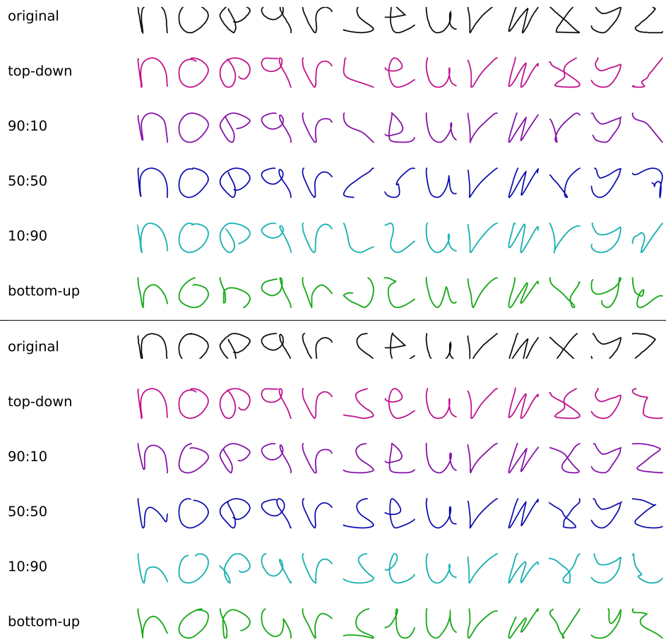
Figure 6: Occluded original input images (either top or bottom occluded) and refilled trajectories, when either using the top-down or bottom-up pathways separately, or a combination of them with equal (50:50) or biased (90:10 and 10:90) weights. The top-down path worked best for this task.
