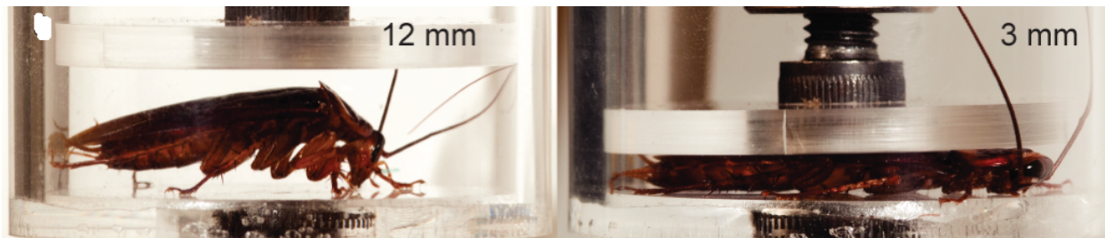
Figure 1.17: Materials testing apparatus with custom built chamber positioned atop load cell to the measure force during cyclic compression (Movie S3).
