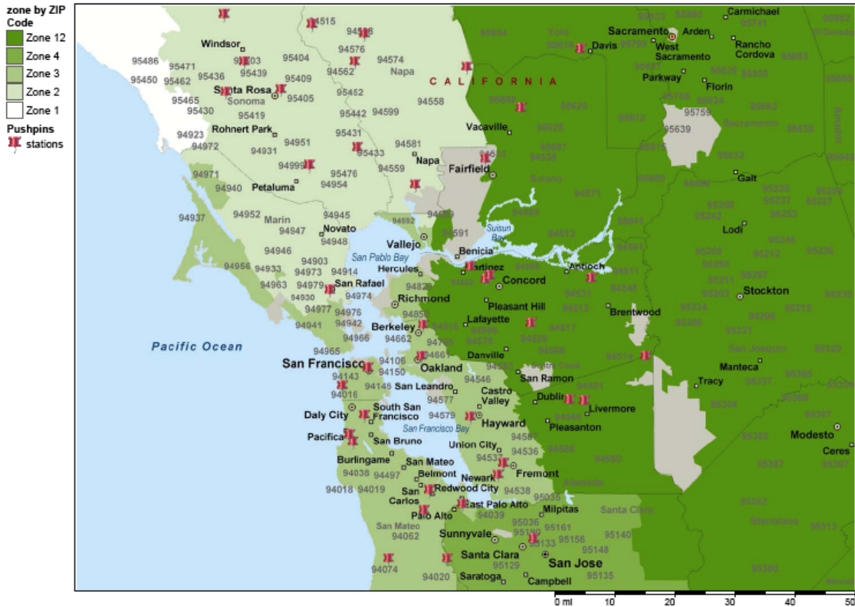
Figure 1. Bay Area California Energy Commission Building Climate Zones (Shaded) and Weather Station Locations (Pins)
