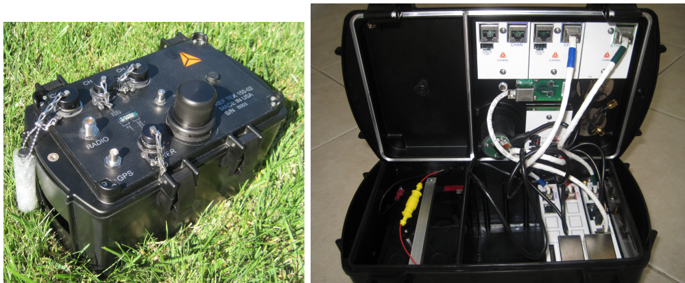
Figure 4.2: GeoNET (RefTek RT155) product photo (a) and internal bays (b)
