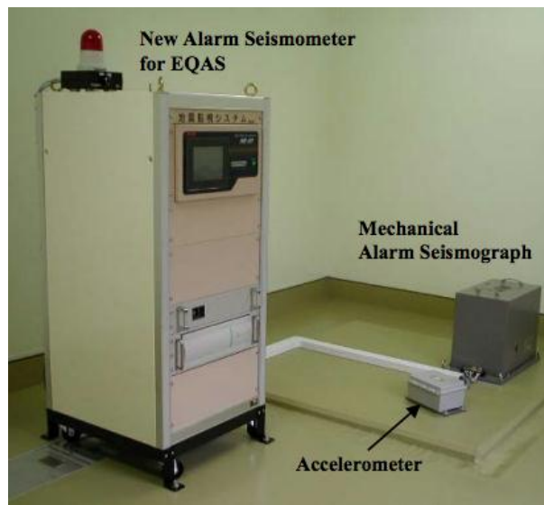
Figure 4: UrEDAS Earthquake Observation Unit [8]
