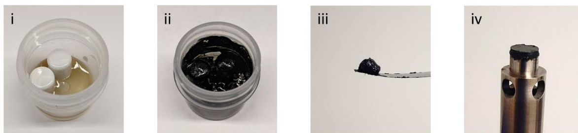
Figure B6 Images of representative sample throughout processing. (i) Bottlebrush polymer with plasticizing monomer in a mixing cup with ceramic cylinders visible directly prior to the addition of CNTs. (ii) Sample from the previous image directly after addition and dispersion of CNTs via centrifugal mixing. (iii) Portion of dispersed CNT sample after adding the rest of the formulation (including crosslinker, catalyst, and monomer, as given in Tables B5–B7), but prior to annealing. (iv) Cured composite sample directly after annealing and successful network formation.
