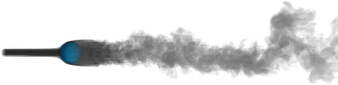
Figure 4.15: Visualization of a passively advected smoke in a flow past a sphere and for a Reynolds number Re = 5,000 .
