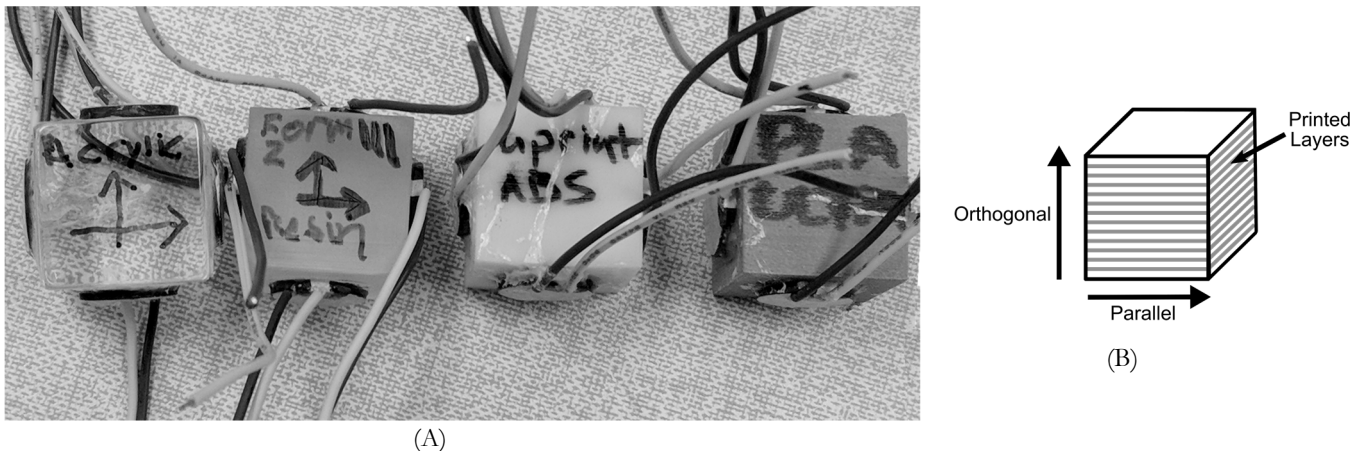
Figure 1. (A) The four types of samples, with the ultrasonic transducers installed, tested in this study. From left to right Acrylic (control), Form 2 Clear Resin, uPrint ABS, and Ultimaker PLA. Coordinate systems indicate wave travel directions parallel or orthogonal to the printed layers, and were drawn on the cubes after printing. (B) The convention used in this study to define the orthogonal and parallel directions of wave travel. The grey lines indicate the 3D printed layers of the sample. When waves travel parallel to the layers they move along the path of a printed layer. When waves travel orthogonally they move through multiple layers.
