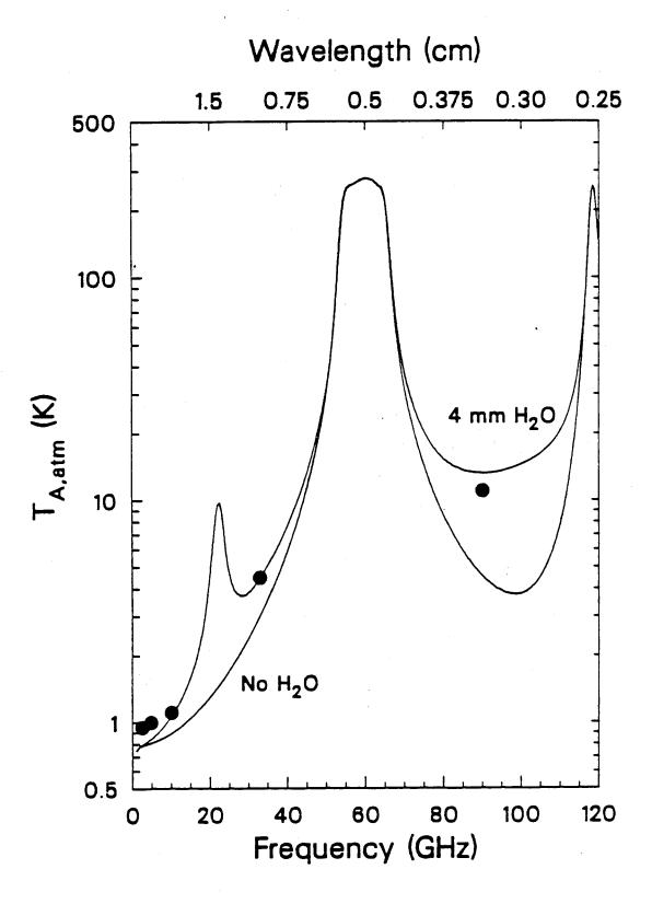
Figure 2: Measured and calculated atmospheric emission at 3800 m altitude of the White Mountain Research Station at Barcroft. Plotted points are our typical measurement values.
