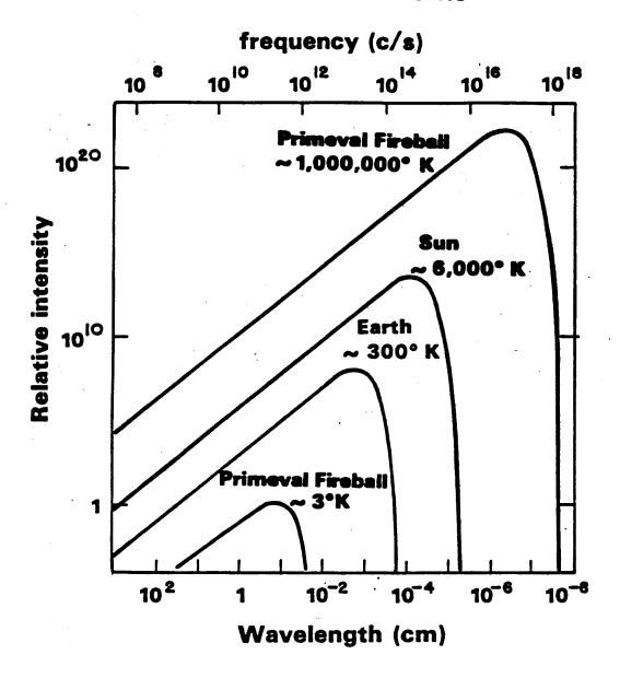
Figure 1: Curves of intensity of radiation versus wavelength (or frequency) for four sample blackbody temperatures.
