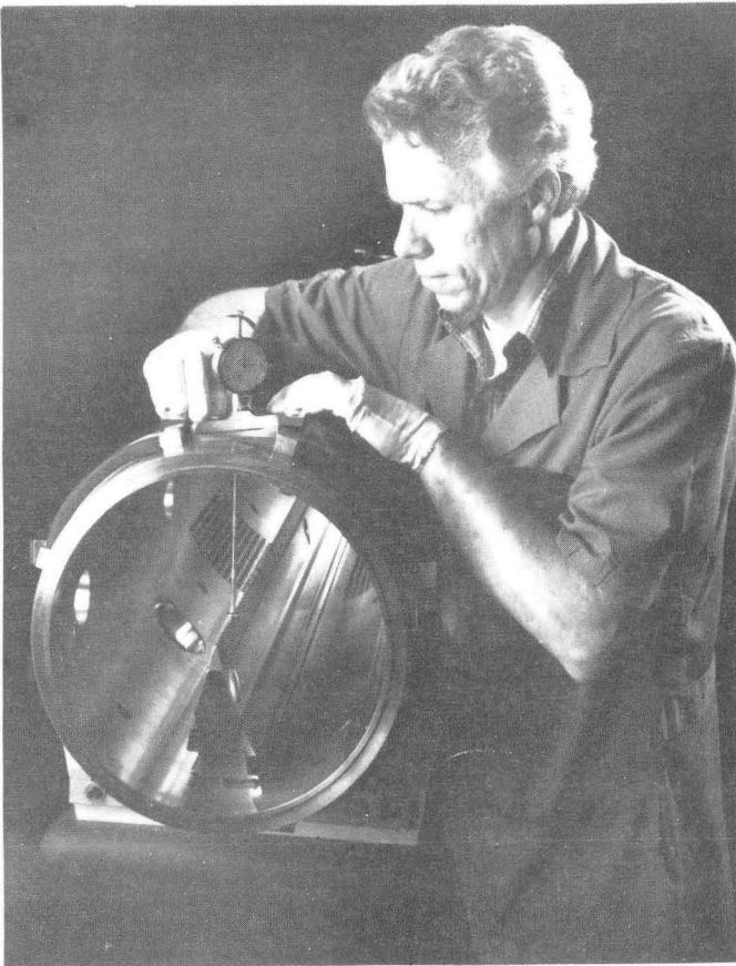
Figure 3: Measuring radial position of vane
