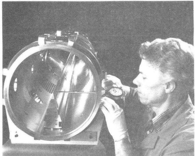
Figure 2: Measuring transverse position of vane
