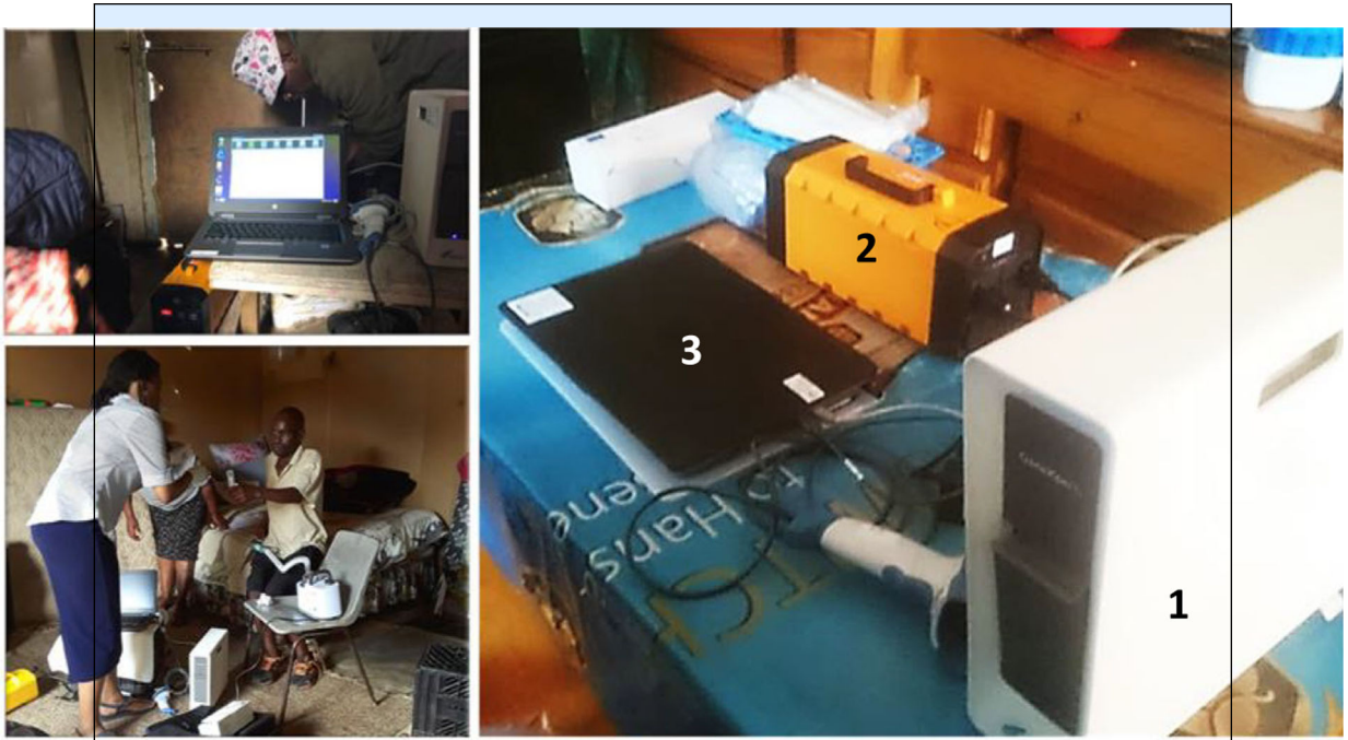
Box 1. Typical home-based testing set-up (floor vs countertops) of the GeneXpert-I single module device. 1 = GX-I device; 2 = UPS portable battery; 3 = standard laptop
