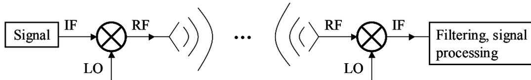
**Figure 1 Schematic of the application of a mixer in an RF communication system**
