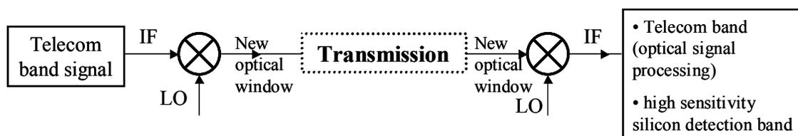
**Figure 3 Optical system architecture that is enabled by optical mixer**
