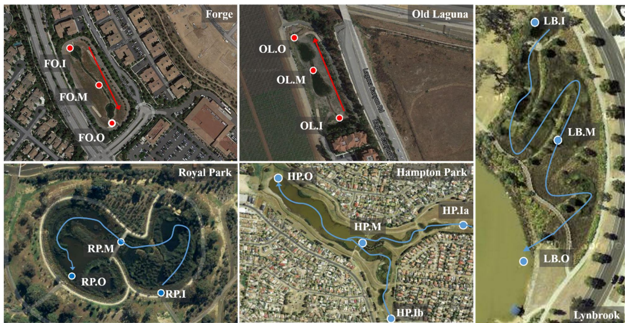
Figure 3-1 Aerial view of constructed stormwater wetlands (CSW) and sampling locations (adapted from Google map, lines show the water flow direction).
