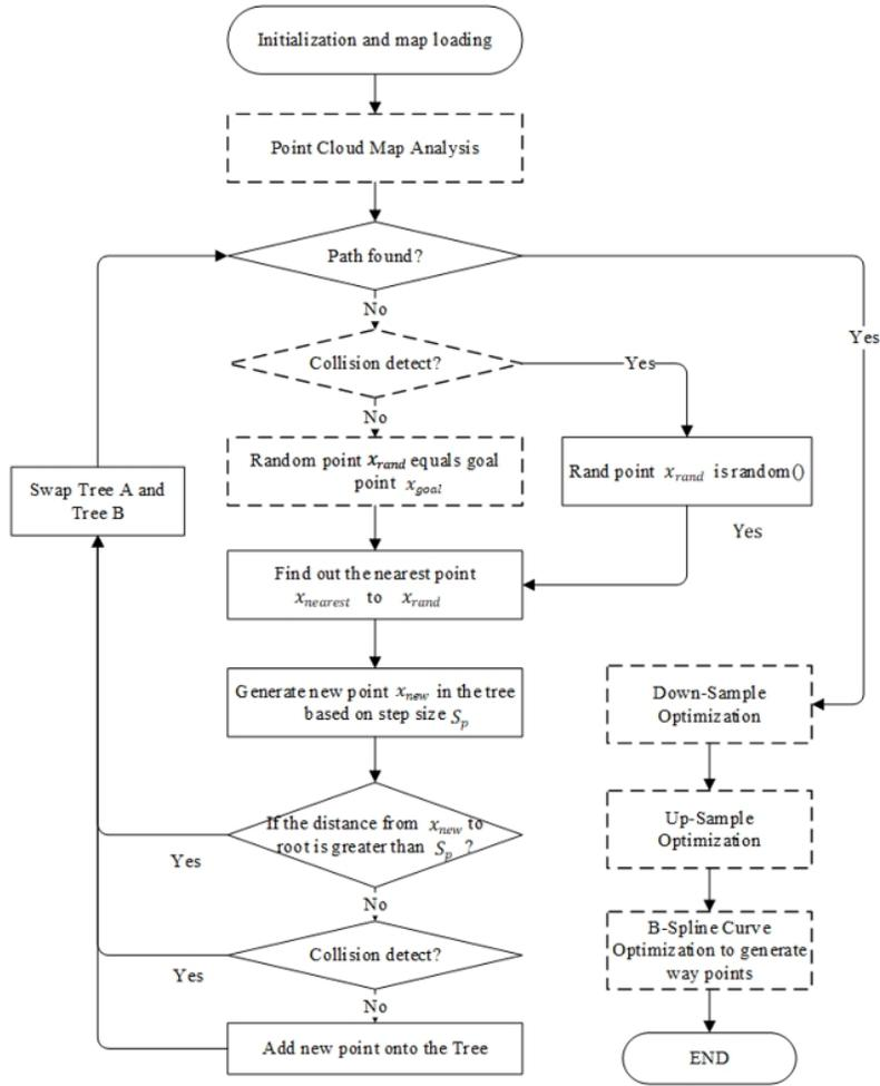
**Figure 3.1:** PT-RRT algorithm workflow
