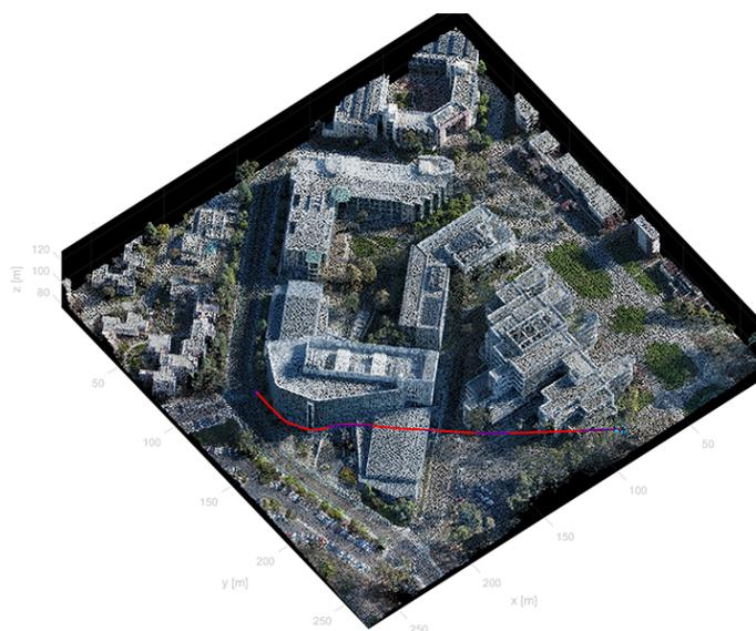
**Figure 1.1:** The blue trajectory is generated by our path planning algorithm and the red trajectory is the real UAVs trajectory after implementing the way-point based close-loop quadrotor control. Video is available at: <https://youtu.be/DEHC7H58QWc>
