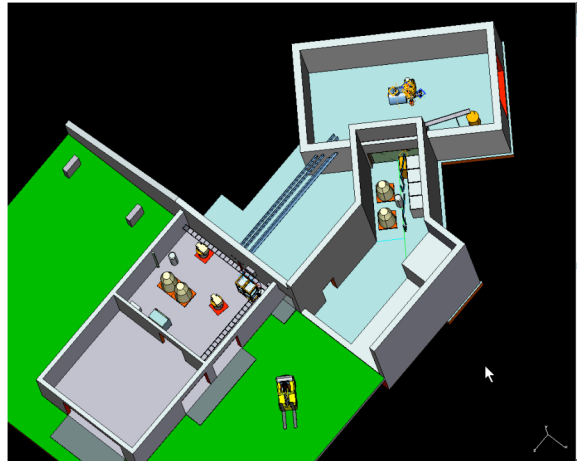
Fig. 1, The MUCOOL Test Area. The experimental area (top) is connected to hydrogen refrigeration equipment (lower left). Beam will enter from top right.
