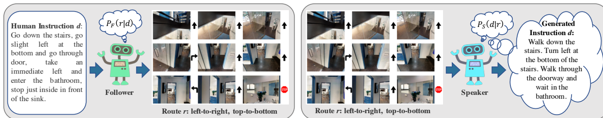
Figure 7.1: The task of vision-and-language navigation is to perform a sequence of actions (navigate through the environment) according to human natural language instructions. Our approach consists of an instruction follower model (left) and a speaker model (right).
