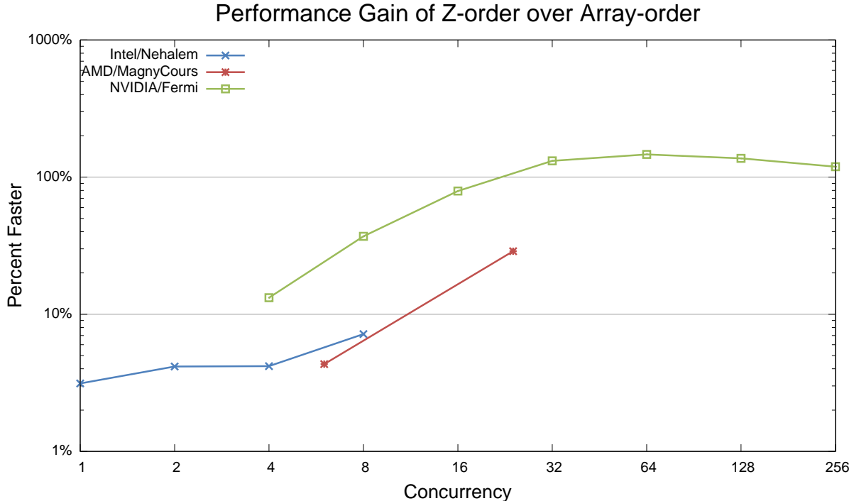
Figure 7: The performance gains (averaged across thread block size, with ERT) from using Z-ordered memory instead of array-ordered increase with concurrency. The gains are most notable on the NVIDIA/Fermi, where we count the number of threads per block as the concurrency.
