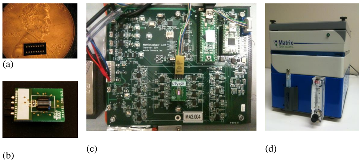
Fig 4.1 Overview of CMUTs and data acquisition. (a) wafer-fabricated CMUTs chip before wire-bonding (b) wire-bonded CMUTs chip (c) data acquisition circuit board (d) Matrix Sensor reader.
