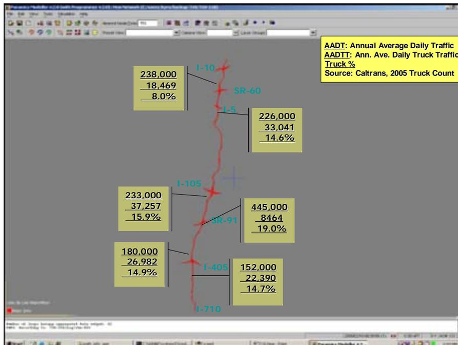
**Figure 3. PARAMICS I-710 network and truck counts based on 2005 data.**
