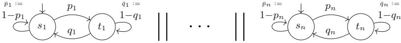
(a) Motivating factory Markov chain with s_i = \llbracket c_i = 0 \rrbracket, t_i = \llbracket c_i = 1 \rrbracket .
