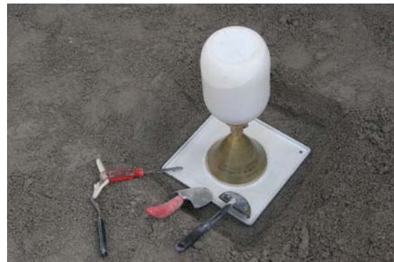
Figure 4.10. Sand cone installed on test pad
