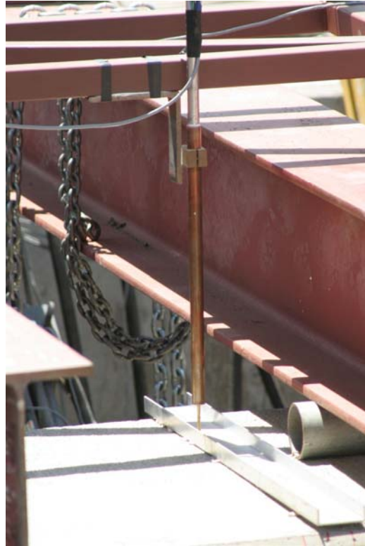
Figure 3.6. Photograph of vertical LVDT at top face of the test specimen
