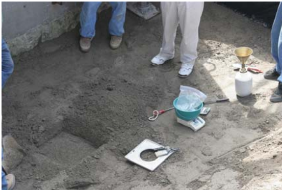
Figure 4.9. Excavation of pad for sand cone testing in compacted backfill
