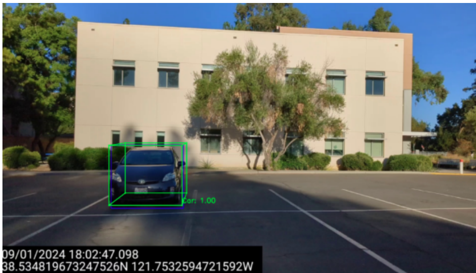
(b) 3D bounding box estimation of a vehicle using MonoDTR, demonstrating depth estimation and spatial localization in the scene.
