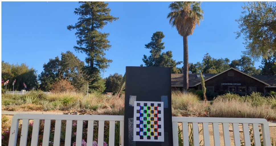
(b) Detected corners on the chess board pattern, marked with colored dots, illustrating successful corner detection for camera calibration.
