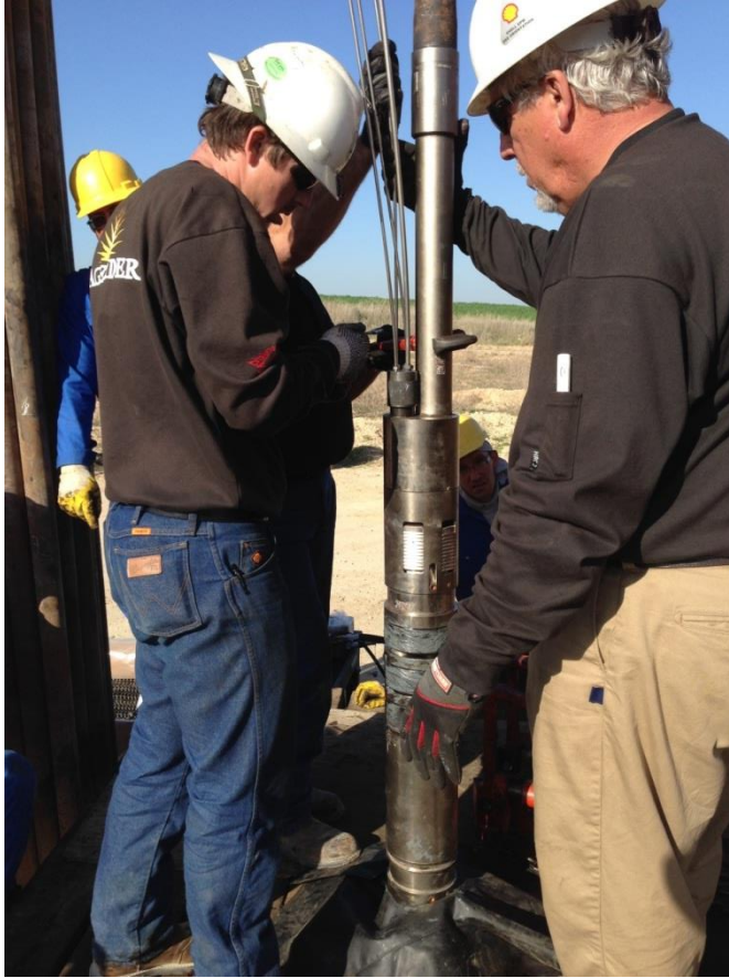
Fig. 8.4.2 D&L dual-mandrel hydraulic set packer with short string fitted with adapter to seal around control lines using compression fittings.
