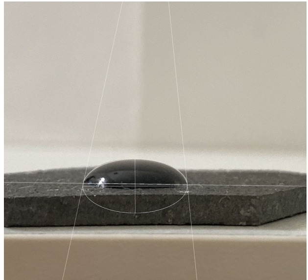
Figure 5. User controlled 10ml syringe to dispense distilled water droplet on cast iron samples.
