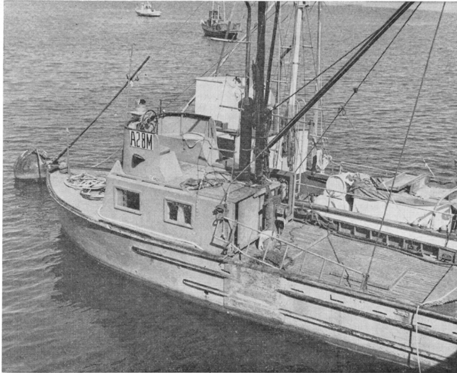
FIGURE 59. A pickup boat used to collect pink abalones from divers working the Channel Islands. These boats are about 50 feet long and can haul several tons of abalones per trip. Photo by Glen Bickford, 1959.
