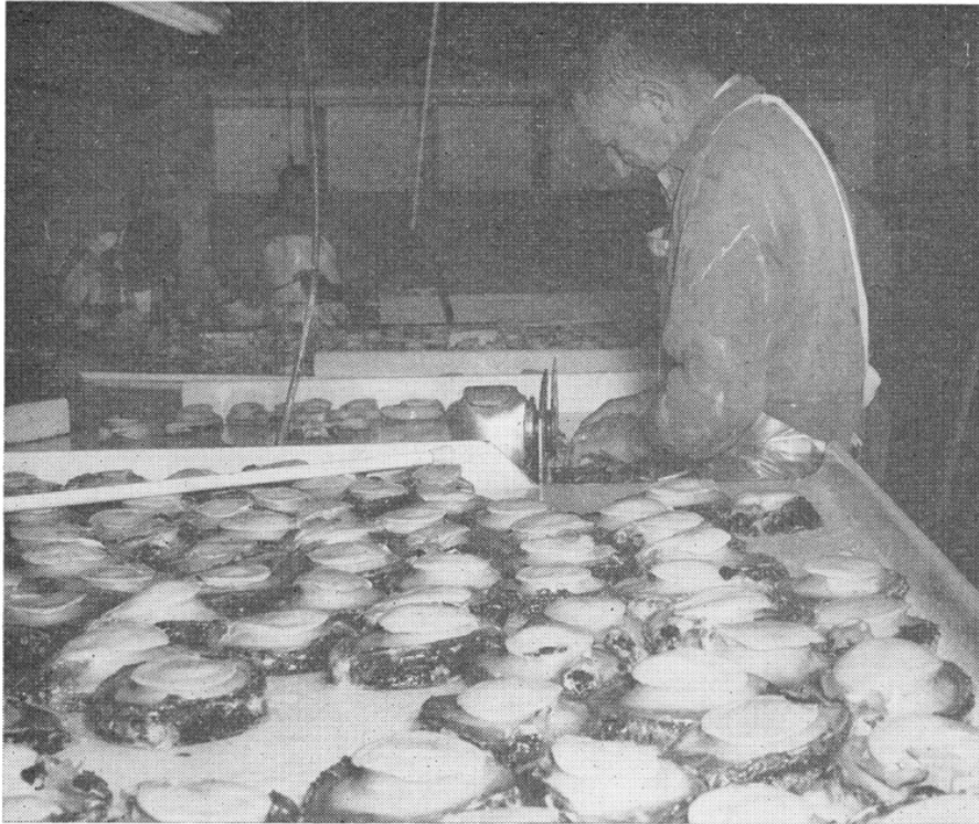
FIGURE 46. Preliminary trimming with a slicing machine removes most of the epipodium containing the black pigment. This process was formerly done by hand using a knife. Photo by Glen Bickford, 1960.
