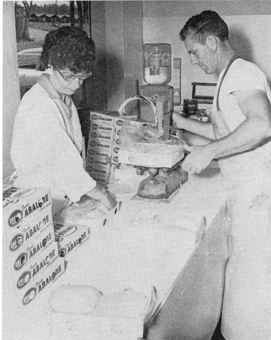
FIGURE 51. The pounded steaks are graded according to quality (color) and size, packed in cartons, weighed and quick frozen. Photo by Glen Bickford, 1960.
