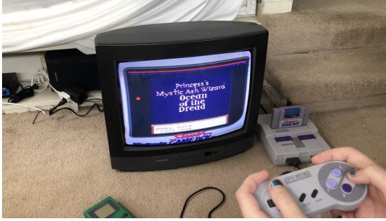
Fig. 1. The generated game Princess's Mystic Ash Wizard: Ocean of the Dread , running on the Super Nintendo, via the Super Game Boy cartridge. The Super Game Boy is an official Nintendo peripheral that allows Game Boy cartridges to be played on a Super Nintendo Entertainment System, and is commonly used for streaming Game Boy video, due to the original Game Boy lacking a video out.
