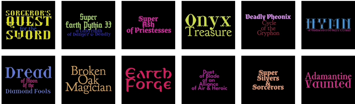
Fig. 5. A selection of title screens generated by the project. Titles are generated via a Tracery grammar, which is then rendered into the title font. The title image layout is resized with seam carving, which both rearranges the elements for better layout in the design and sets the image ratio to match the Game Boy screen resolution.
