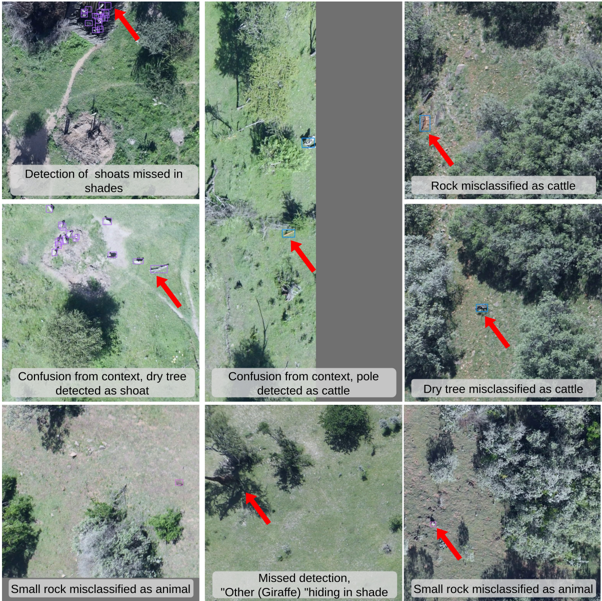
Figure B.2: Failure cases. The animals hiding in the shade are difficult to detect. Additional examples of misclassification also provided.
