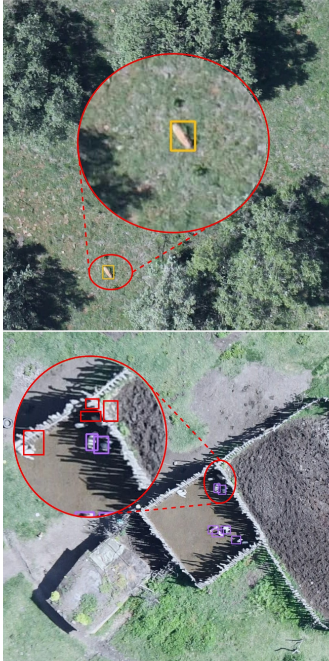
Figure 4.6: Failure cases. Left shows an example where animals are occluded by shadows and are difficult to detect. Right shows an example of rock detected as an impala, emphasizing the difficulty in differentiating objects in the image from animals of interest.
