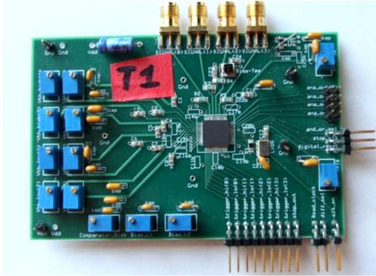
Figure 3.2: Picture of the SST Test Board: Constant Sampling Frequency
