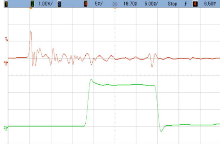
Figure 3.16: Oscilloscope Screenshot Showing the Trigger Sensitivity of the SST Chip
