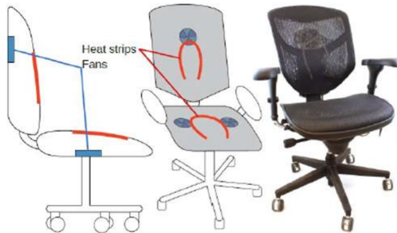
Figure 7: The Personal Comfort System chair with heating strips and fans for cooling.
