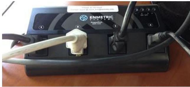
Figure 8: Enmetric Power Port plug load control and monitoring system.
