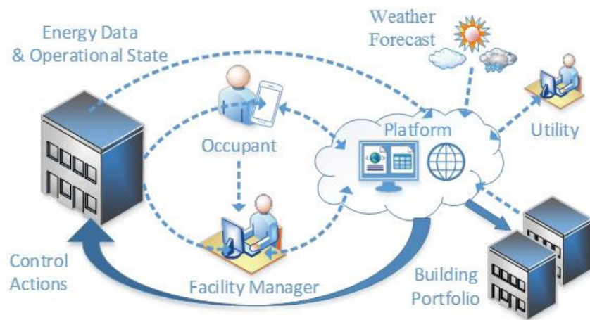
Figure 1. Data flow and control actions in an intelligent energy management system
