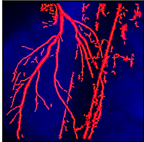
Figure 11.b: Results after initial segmentation and expansion. Red areas are extracted regions. Green points are the corresponding center points.
