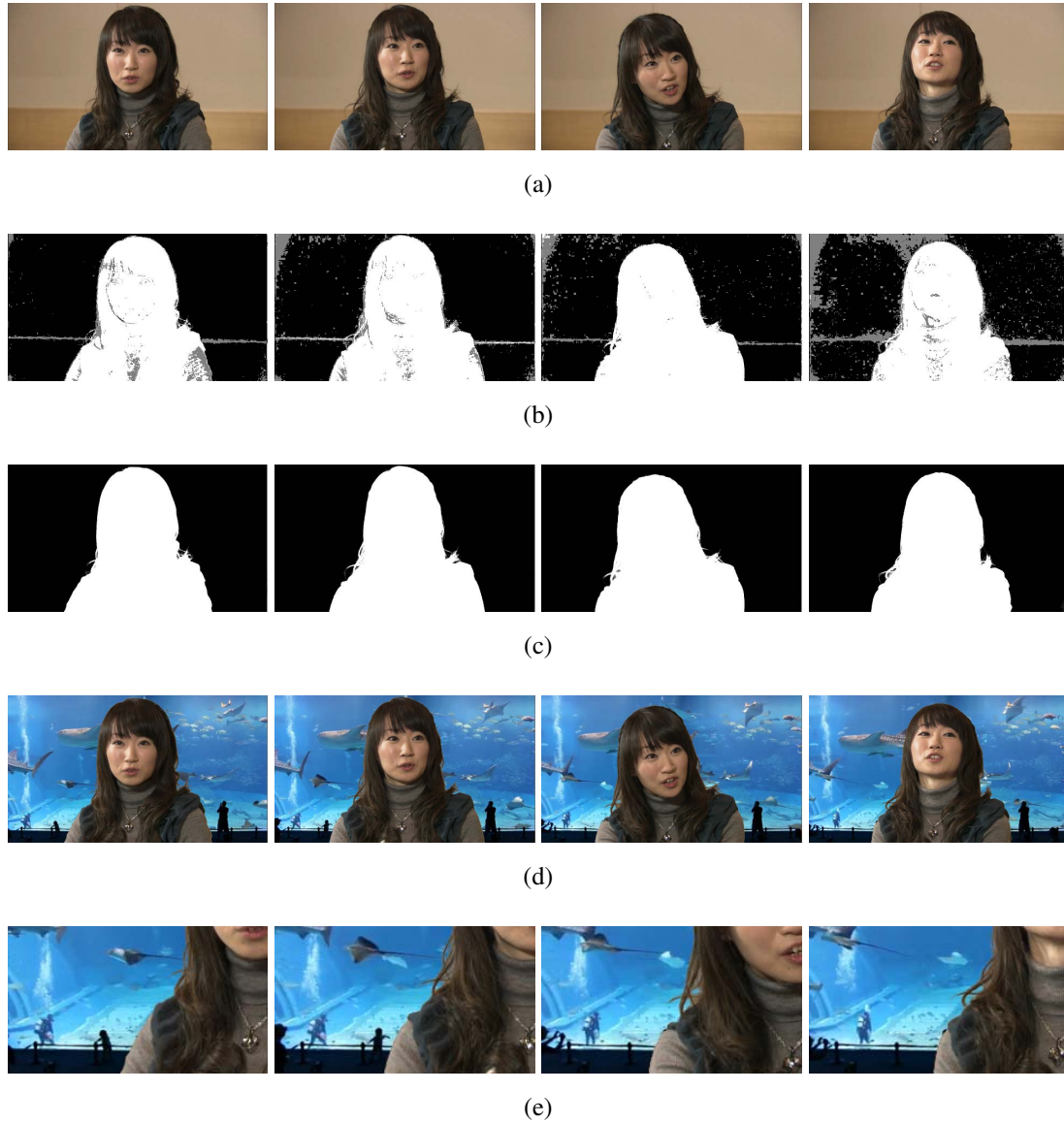
Figure 5.2. Results of Nana sequence: (a) original frames; (b) trimaps; (c) alpha mattes; (d) composites; and, (e) zoomed-in areas of the composites.
