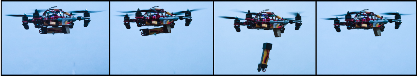
Fig. 6. Sequence of images from the two-stage flight experiment. From left to right: (a) Quadcopter hovers using only first-stage battery. (b) First-stage battery is depleted. Quadcopter starts using second-stage battery. The detaching motor is simultaneously activated to disengage the bolt. First stage is about to fall. (c) First stage is ejected and falls towards the ground. (d) Quadcopter continues hovering using the second-stage battery, with reduced mass and power consumption. Note: We have not attached a parachute in this case to clearly show how the staging works. The first stage fall is broken softly by a net below the quadcopter. In real-life settings, it is advised to use some fall breaking mechanism to not damage the energy source or any property (for e.g. by using a parachute as shown in Fig. 1). All reported experimental flight times and plots use a parachute in the two-stage case.
