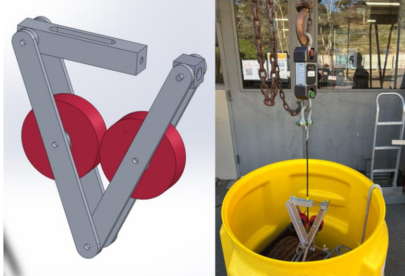
Figure 6: Pinch-roller model and coefficient of friction test setup without water. Dynamometer forces were recorded as the hoist pulled the wire section out of the jig.
