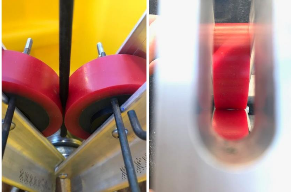
A 1: Inelastic deformation of the 95a polyurethane wheels in the pinch roller from friction tests. The deformation introduced error in the COF results since the normal force calculation assumed only elastic deformation. The effect caused the wire to slip at lower tensions between tests.
