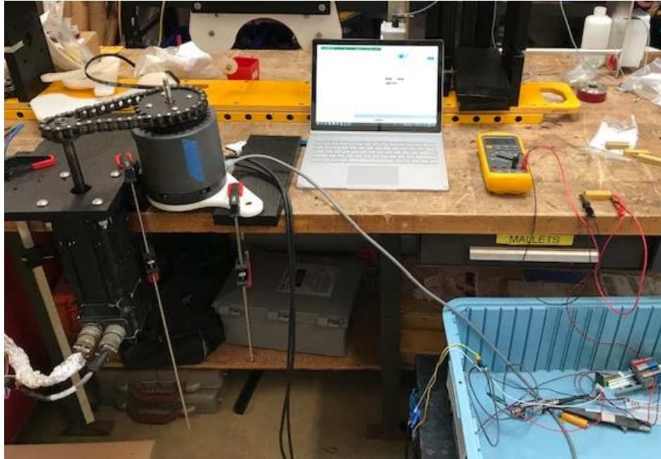
Figure 14: Power Curve test bench setup with the driving motor, generator, Elmo Harmonica on the laptop, multimeter, and load resistor (left to right).
