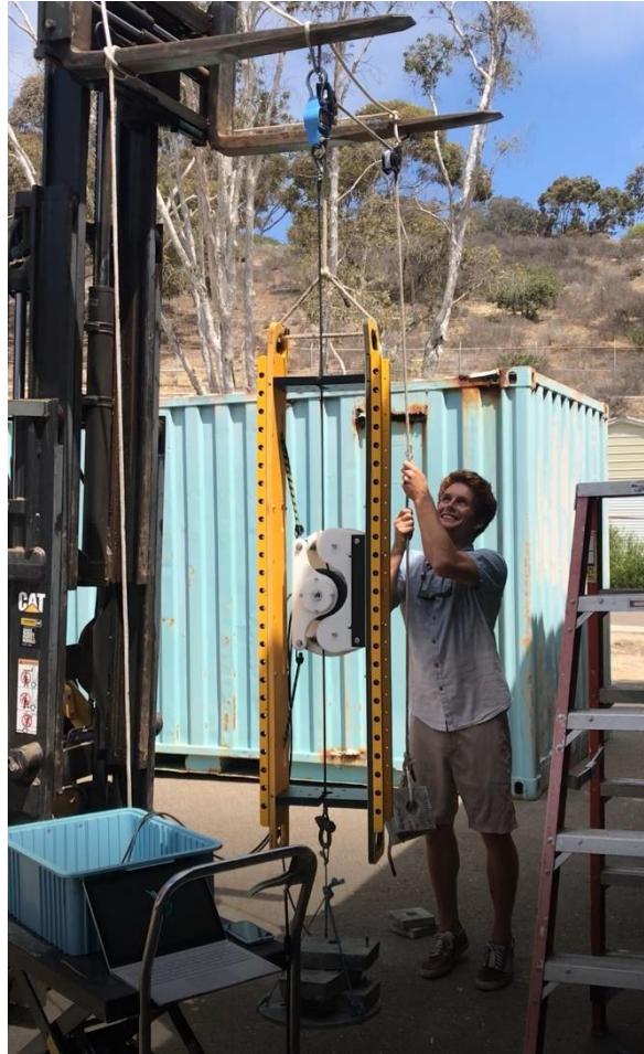
Figure 17: Photograph of dry test set-up courtesy of Tobi. The Livewire was moved with a counter-weighted offset rope, while the change in wire tension was measured with a dynamometer.
