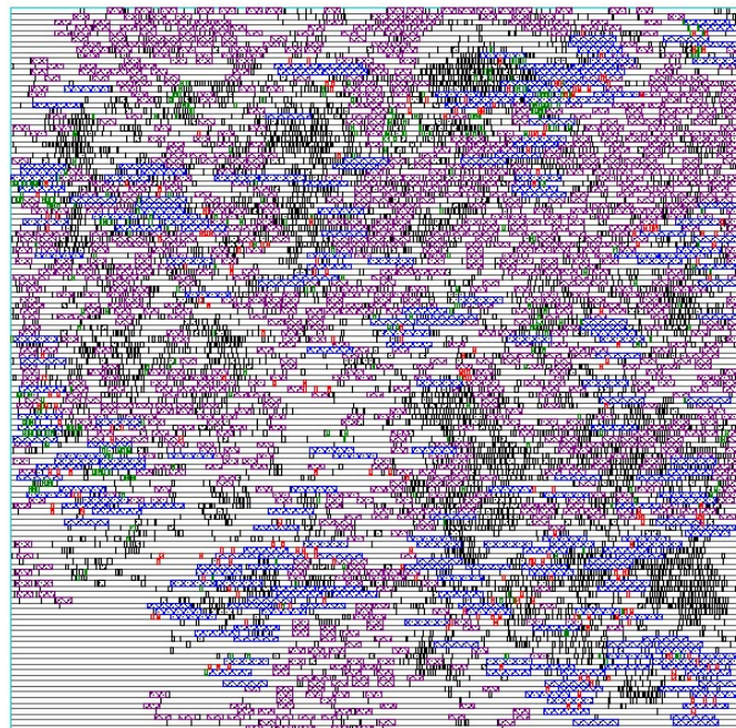
Figure 3.41: Layout of CombOpt result for the SPU testcase with 3\sigma corner. Razor flip-flops are in blue; conventional flip-flops are in purple; OR gates are in red; and hold buffers are in green.
