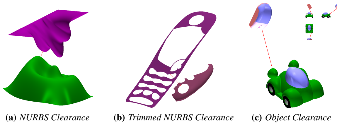
Figure 6.1: Minimum distance/closest point computations between NURBS surfaces and complex CAD models accelerated using the GPU.
