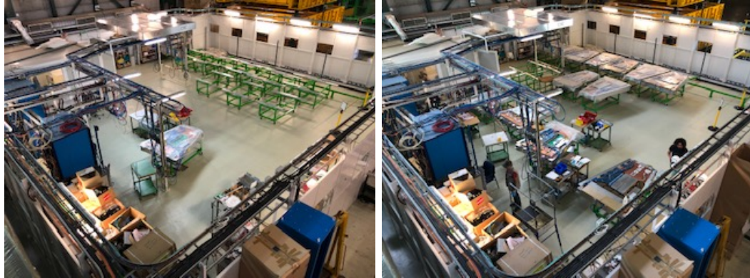
Figure C.1: (left) The SX5 Surface Lab with mostly empty chamber tables, in Green. Chambers follow a zig-zag pattern, being refurbished near the middle-right before proceeding to the FAST test stands to the left, and then the Long Term Test stand (LTT) under the fume hood in the top of the image and Fig. C.2. (right) For most of the production, the lab was filled, with chambers being actively refurbished, tested, or awaiting delivery to the Experiment Cavern on tables.
