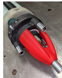
Fig. 10. Laser tracker targets: these are mounted on the bearing block at one end of the coil.
